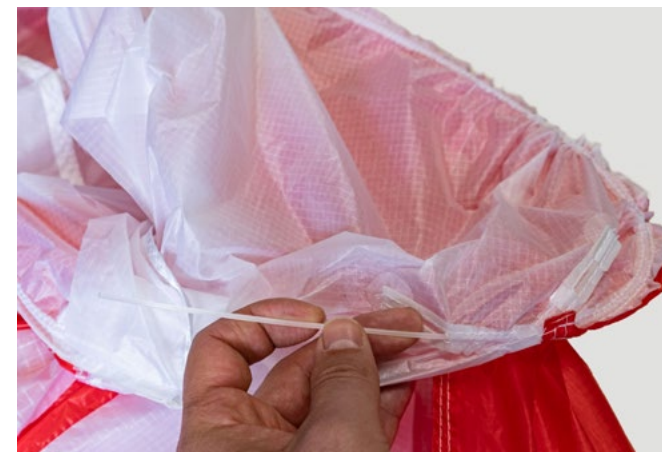
Pull the rod out. Compare the old rod with the new material and cut it to the correct length. Insert the new piece into the pocket, ensuring both ends of the rod are fully anchored in the small pockets at both ends. (Photo 3)
